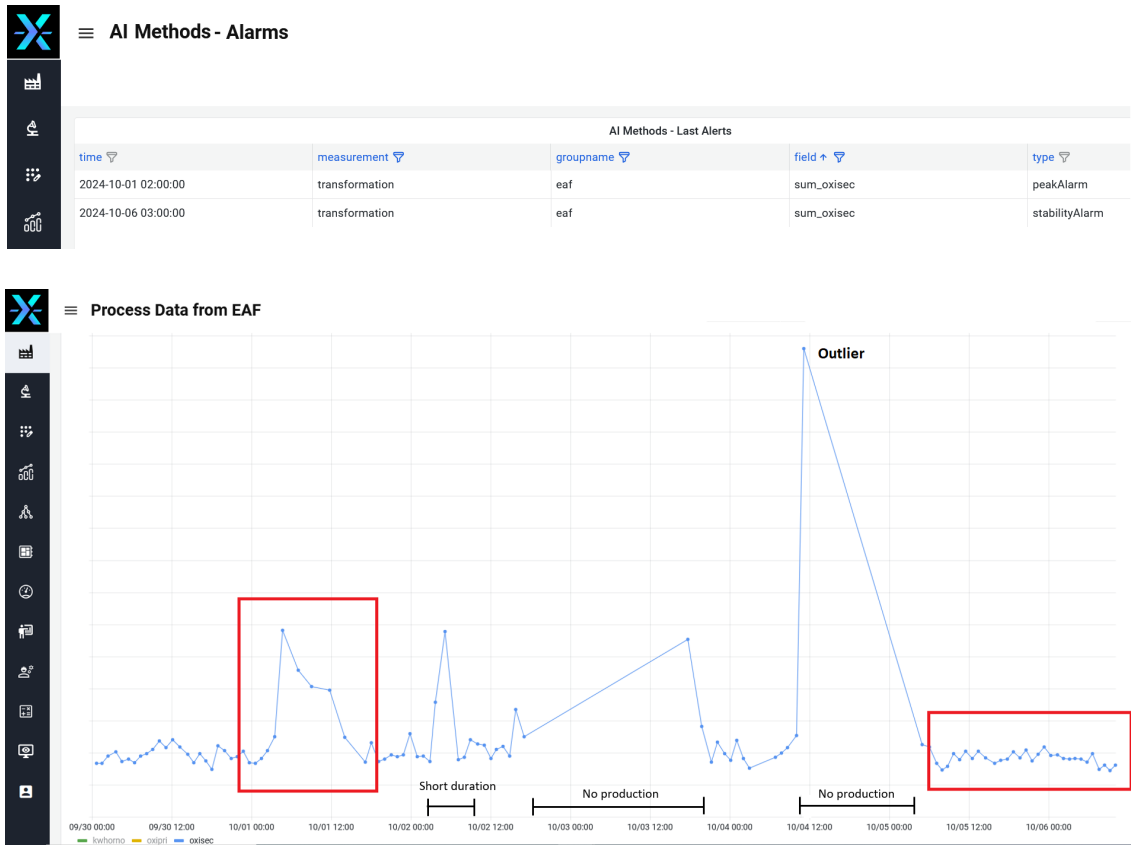
Figure 7. The alarms generated by the AI methods for the cumulative amount of secondary oxygen in the transformation stage are shown in the upper plot. The raw data for the cumulative amount of secondary oxygen are shown in the lower graph, with the alarm-triggering periods indicated by red rectangles.
